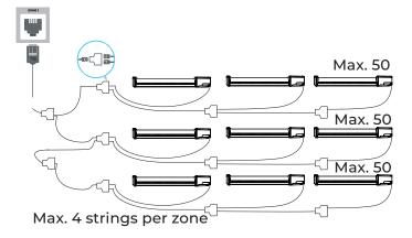
**Attention**: ONLY use cables supplied by Dutch Lighting Innovations. Each zone must have a single wattage/type of fixture connected to it.
